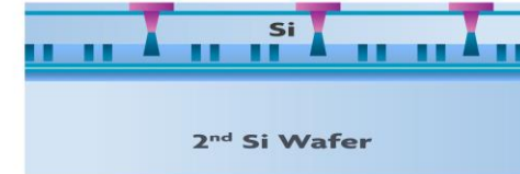
Backside single Cu damascene metallization
