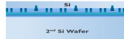
Selective Si etch and removal of the buffer layer
