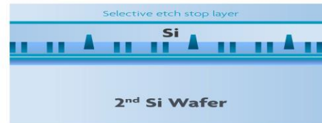
Wafer grinding and thinning to < 5\mu\text{m}
